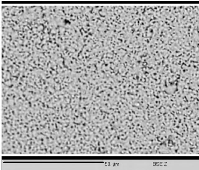
Fig. 5. Back-scattered image for the nominal composition \text{Ce}_{0.15}\text{Y}_{0.595}\text{Nd}_{0.255}\text{O}_{1.575} . The dark pots correspond to the pores as confirmed by EDX analysis.
